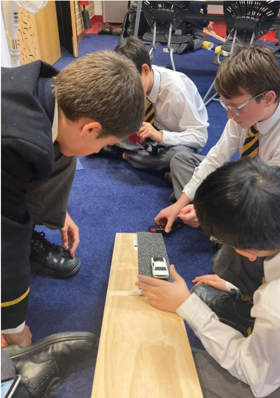
Boys testing the speed of model cars on various surfaces to understand the forces of friction
